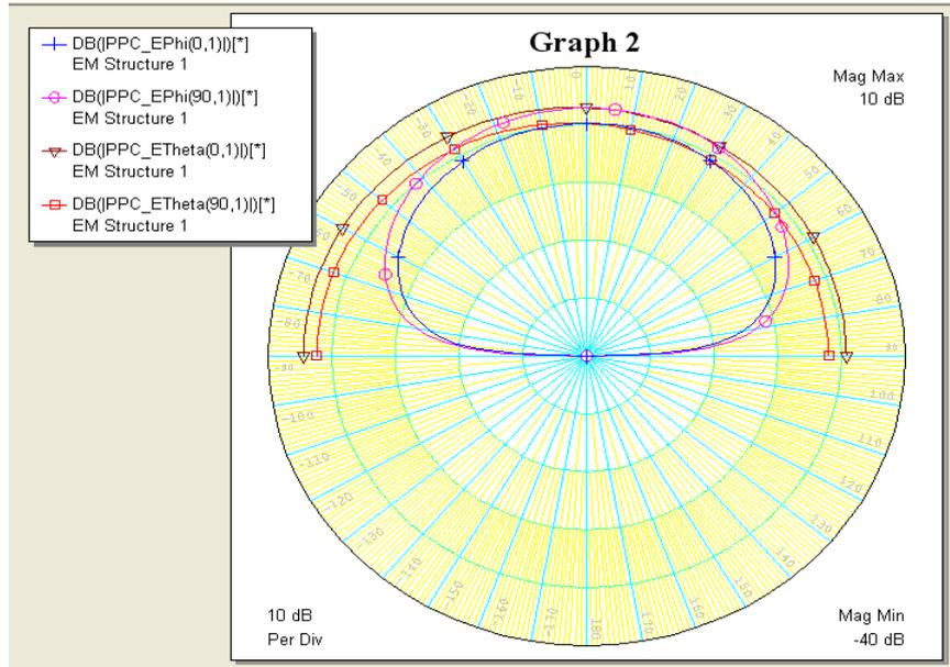
Figure 7. Simulated radiation pattern in terms of (E –CO, E-CROSS, H-CO, H-CROSS)
