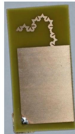
(b). Antenna prototype (fabricated)
