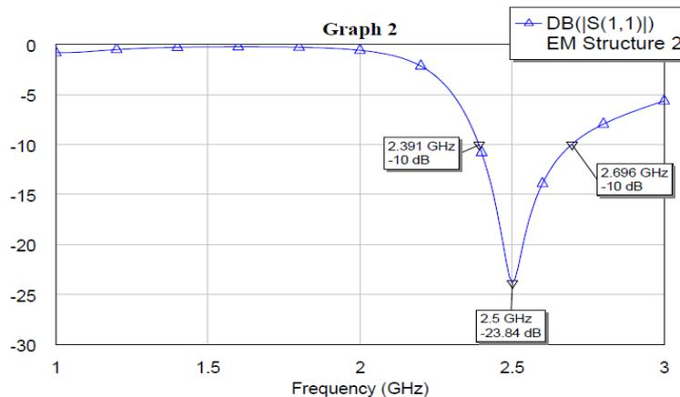
Figure . 4 ( $S_{11}$ ) simulation result of the antenna fed via coaxial probe
